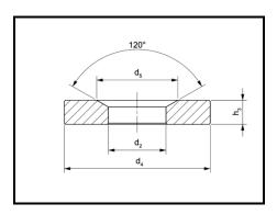
Compared to conical seats form D, due to its solid construction conical seats form G are specially qualified for use with slotted holes or for levelling out uneven ground.
